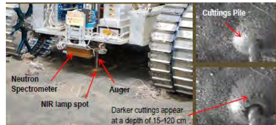
Figure 1. The RESOLVE Payload on the Artemis Jr. rover: Shown is an augering activity with the NIR lamp illuminating the drill spot the view from the Drill Camera.
