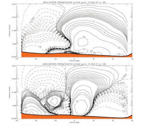
NASA-Ames GCM simulations of the mass stream function based on 10 sols of data from Ls=185 show a significant difference in the strucutre of the Hadley circulation. Dust forcing in Hellas is perturbing the circulation, resulting in a longitudinally dependent disturbance: in the eastern hemisphere, a symmetric Hadley cell extends from the equator to each pole – stronger and broader than usual. Sinking motion associated with the descending branch causes compressional heating.
